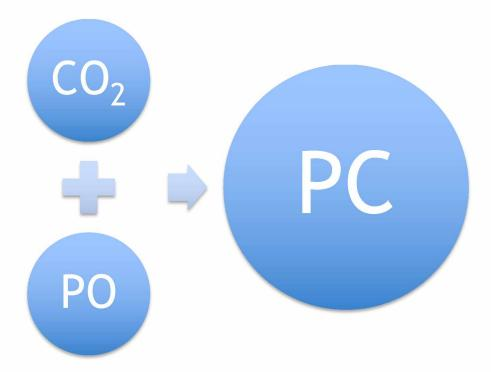
Both  $CO_2$  and PO are fed to a reactor. The reactor operates near atmospheric pressure with a temperature of 170°C. Under these conditions a catalyst is required in order to produce PC. In time, the catalyst deactivates and can be regenerated with OctBr.
