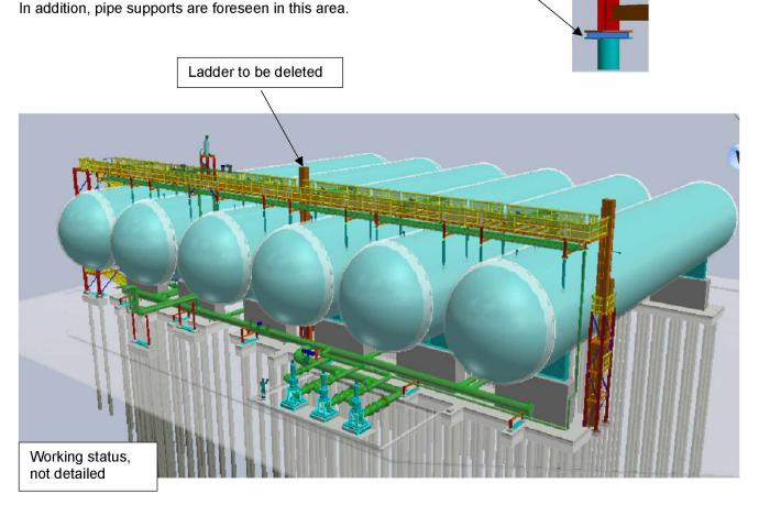
CO2 storage tanks are supported on two saddles (fixed and sliding saddle). Saddles are supported by large concrete pedestals on common foundation beam and on piles.
