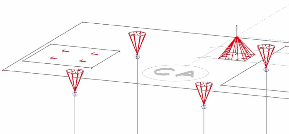
The same technic is used for the columnsupports. This is also done to insure no unwanted stresses due to local points are applied.
