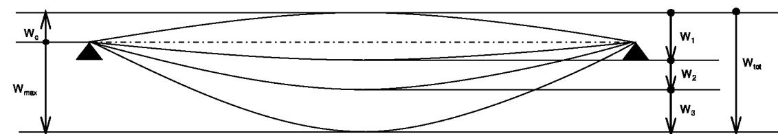
$W_c$  = The calculated value of the camber for the structural component in serviceability limit state (SLS);
