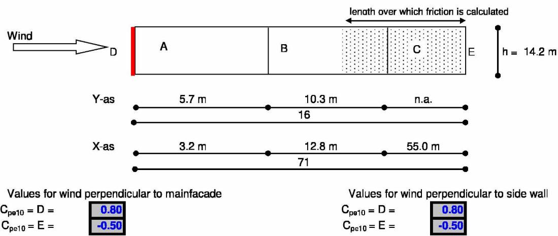
Structure is considered as a big beam on supports. Windfactor is considered as 0.8 + - 0.7 = 1.5
