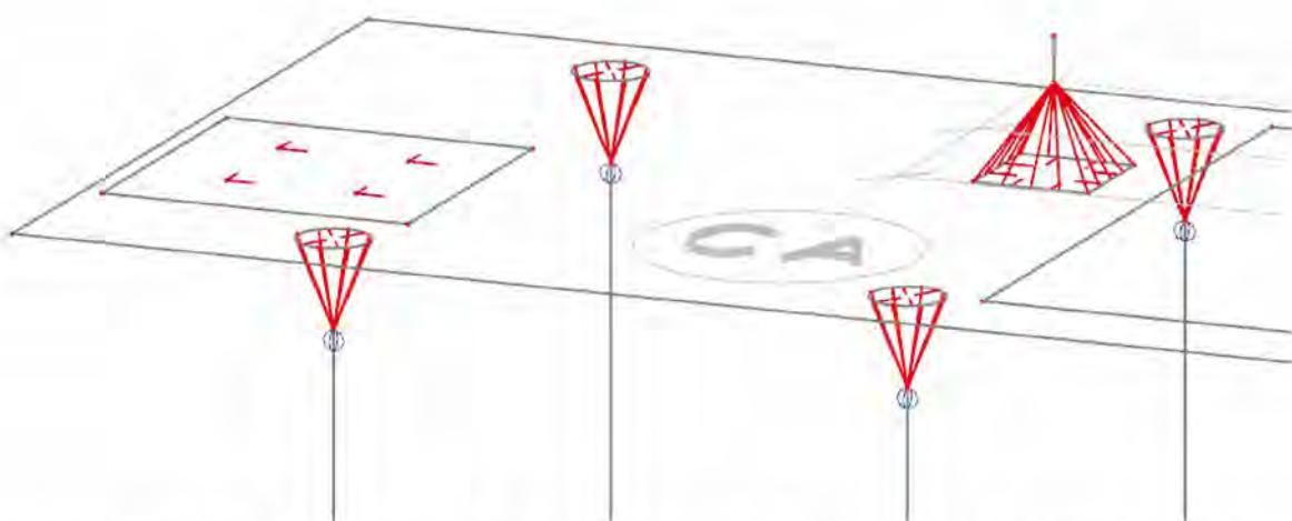
The same technique is used for the columnsupports. This is also done to insure no unwanted stresses due to local points are applied.
