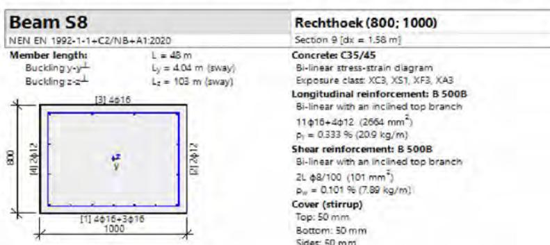
Based on this a first rebar design is made which commutes to = 48.7 kg/m $^3$
